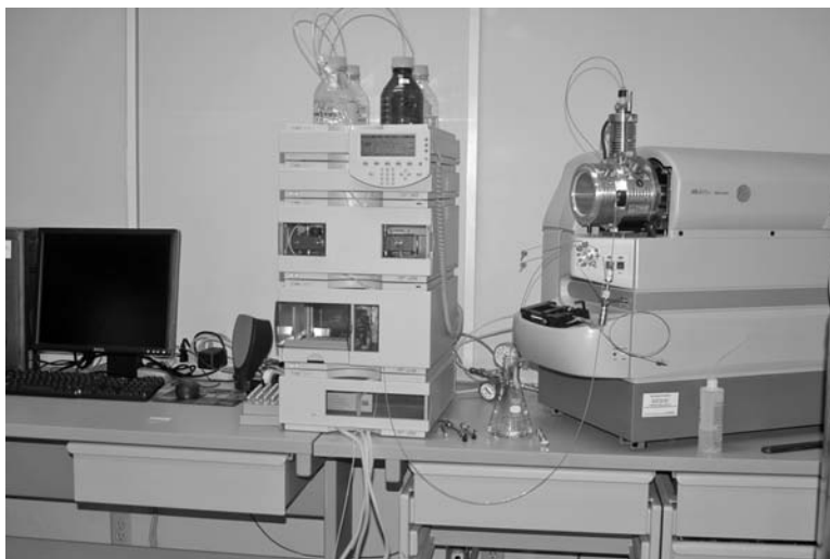
Figure 4.4 A view of one of the many types of analytical instruments (liquid chromatography–mass spectrometry analyzer) in the toxicology laboratory.
