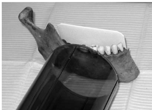
Figure 10.2 Setup for exposing a postmortem radiograph. Proper projection geometry is critical whether using film or digital sensors.
