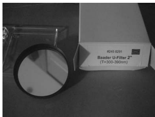
Figure 11.22 The Baader Venus UV filter used for either film-based or digital UV photography.
