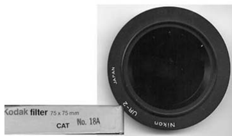
Figure 11.21 The Kodak Wratten 18-A filter used for film UV photography.
