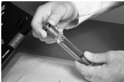
Figure 7.3 Preparing to pulverize a whole tooth in a freezer mill with liquid nitrogen by encasing the tooth in a sterile polycarbonate tube sealed with two metal anvils, including a ferromagnetic plunger. (Courtesy of the BOLD Forensic Laboratory at UBC.)
