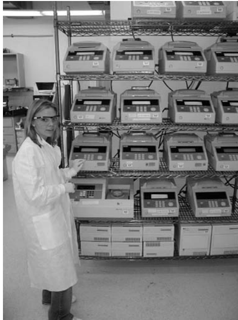
Figure 7.5 A bank of thermal cyclers used to perform PCRs on forensic samples in a high-throughput forensic DNA laboratory. (Courtesy of the Armed Forces DNA Identification Laboratory.)
